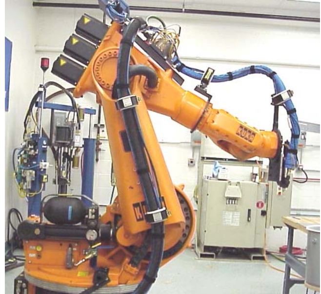
Modified FS dressout on KUKA KR210 with Axis 1 to Axis 3 additional dress
